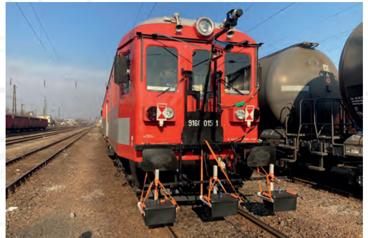
A GPR measuring system mounted on a measuring train
