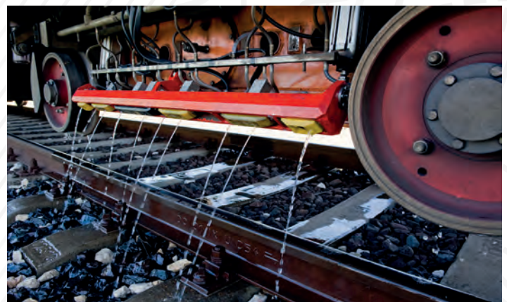
Measuring bogie with ultrasonic inspection heads
