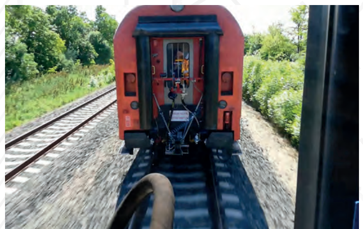
Slip test of an IC coach
